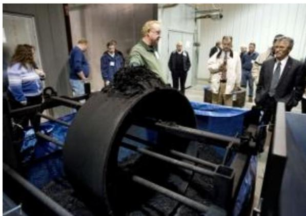
Harvey Buhr points out the powder residue that remains after a solid tire that went through the process after the oil and gas were removed. Buhr, CEO of Hitec LLC, has brought his process of recycling tires into four different components to RDH Tire and Retread company, to make RDH Environmental. Photo by Jon C. Lakey, Salisbury Post.
