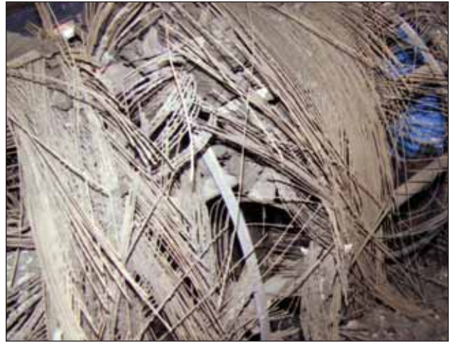
Three 235R25 scrap tires after processing.
