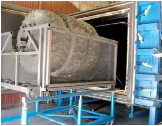
Three 235R25 scrap tires being loaded into the Hitec unit.
